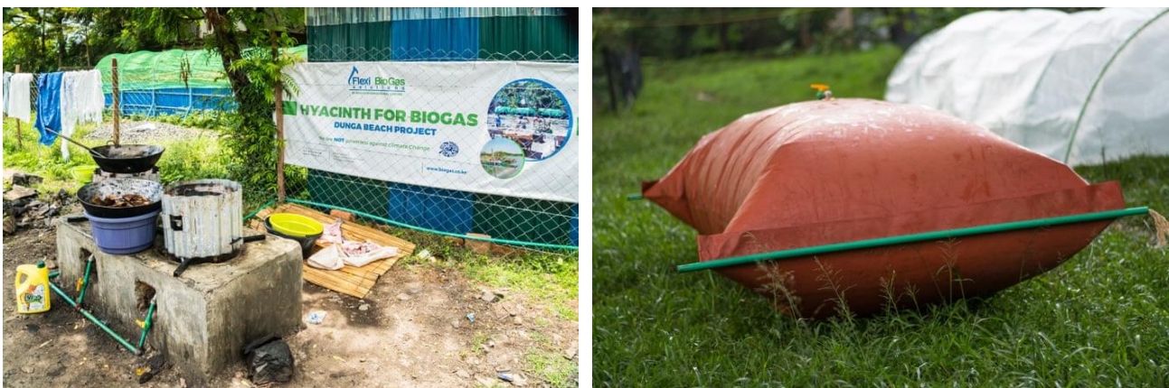
Fig. 45. Demonstrating cooking with Biogas from food waste, and the Methane gas container from Flexi Biogas BG5 using PVC tarpaulin material. Photos: The Guardian and Flexi Biogas
