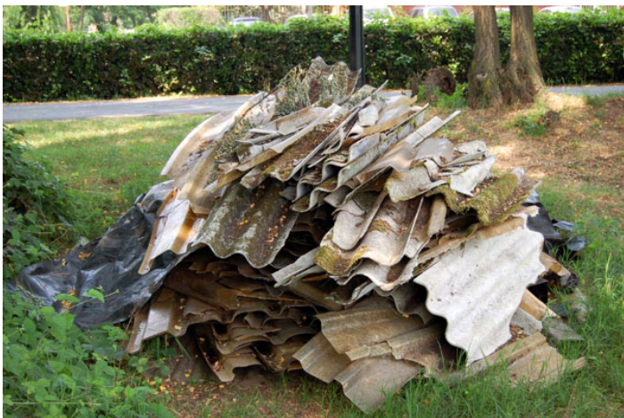
Fig. 36. Broken and old asbestos roofing materials are exposing high risk to public health and must be handled carefully and in an environmentally sound manner. Photo: Kenya CIC
