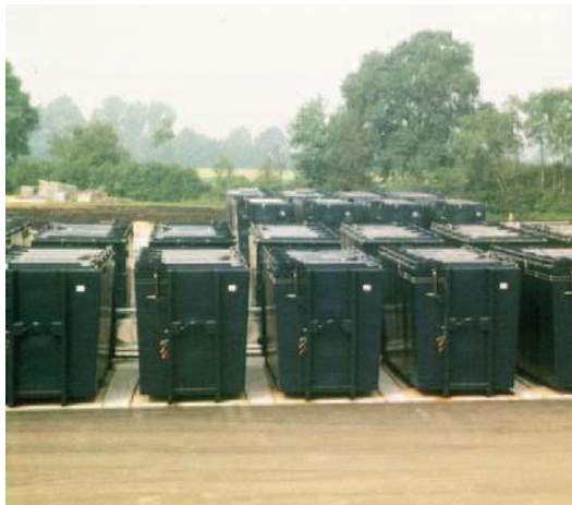
Figure 4.1b: Container composting with controlled aeration (Photo by Ina Körner, courtesy Hamburg University of Technology).
