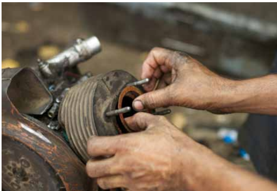
Replacing an asbestos gasket, © ROCA/GAAA
