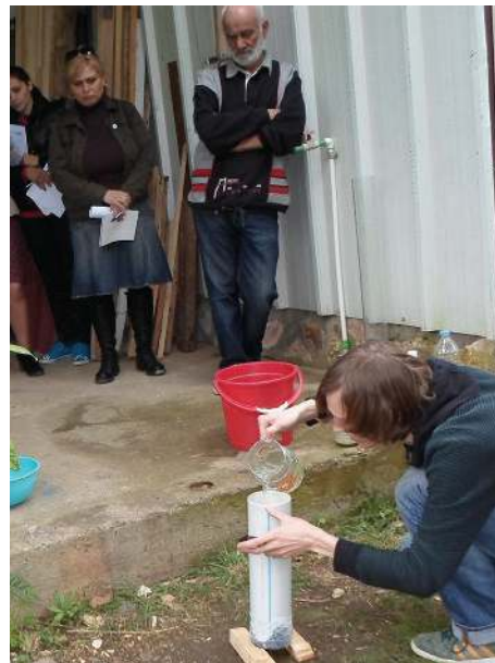
Pictures B and C: Checking the proper sand composition with the kf Test.
