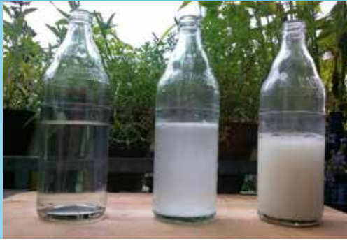
Samples of water turbidity standards with 5, 50 and 500 NTU.
